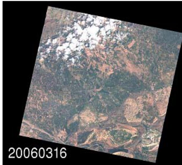
Level 1: Top of the Atmosphere reflectances calibrated & geocoded (orthoimage). Formosat-2 data, 8m ground resolution.
