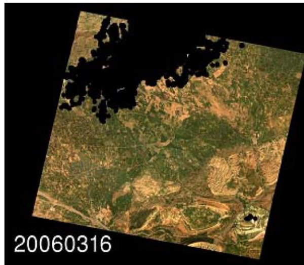
Level 2: Single date surface reflectances after cloud masking and atmospheric correction on level 1 product. Formosat-2 data, 8m ground resolution.
